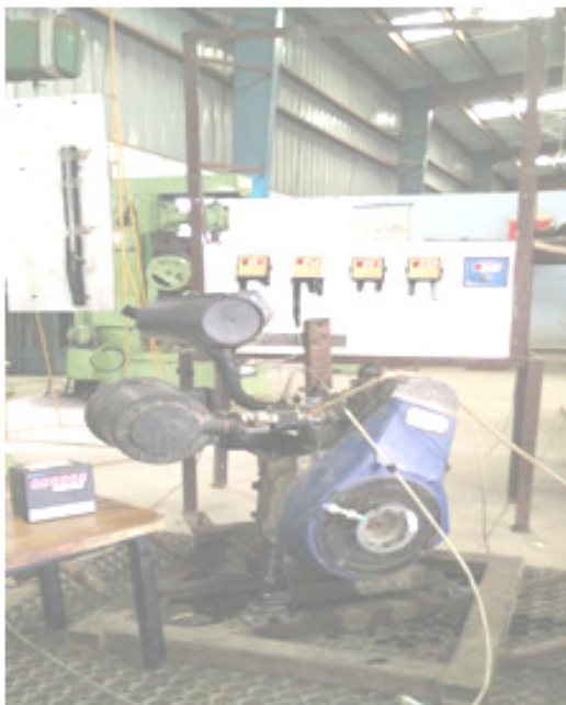
Fig. 3. Test rig for emission and temperature measurement
